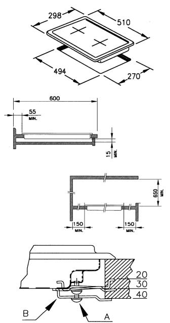
DO NOT overtighten screw 'A', one turn maximum will be sufficient, after correctly fitting shaft 'B' into place (as shown above). Ensure that the supporting surface is perfectly even. Fit the appropriate expanded seal. The hob must not be subjected to strains caused by uneven supporting surfaces.
